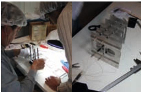
Figure 2: The new imager baffle. Left: being assembled by Gilles Durand, the VISIR project engineer of CEA/DAPNIA. Right: after assembly but before integration into the camera assembly.
