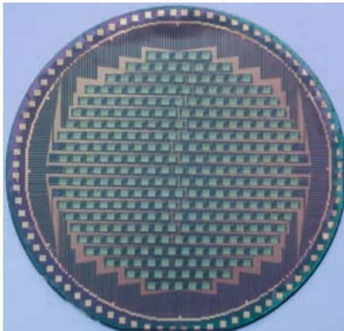
Figure 1: A 'naked' LABOCA silicon wafer. Each small square is a bolometer.
