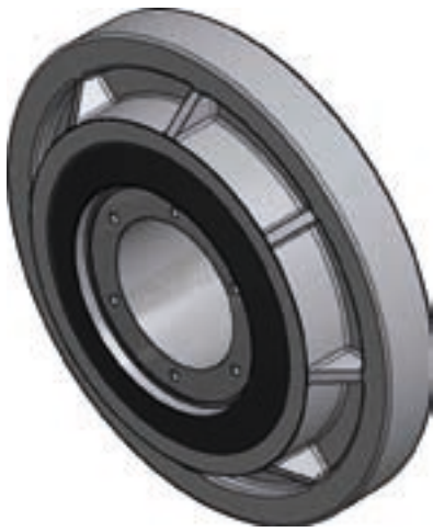
Figure 3: Details of the composite structure of the dome support wheels.
