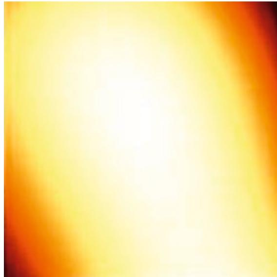
Figure 3: R-band flatfield correction frame.
