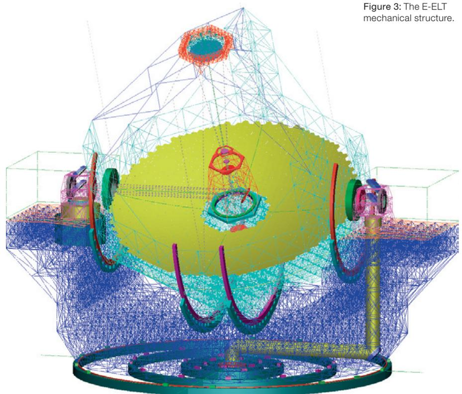
Figure 3: The E-ELT mechanical structure.
