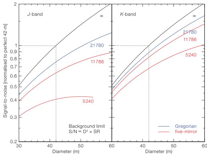
**Figure 6:** Signal-to-noise versus telescope diameter as a function of adaptive optics technology. The numbers of actuators for the options studied are indicated (from top to bottom): perfect AO; 30-mm pitch at the Gregorian secondary; 20- and 30-mm pitch at the five-mirror quaternary.
