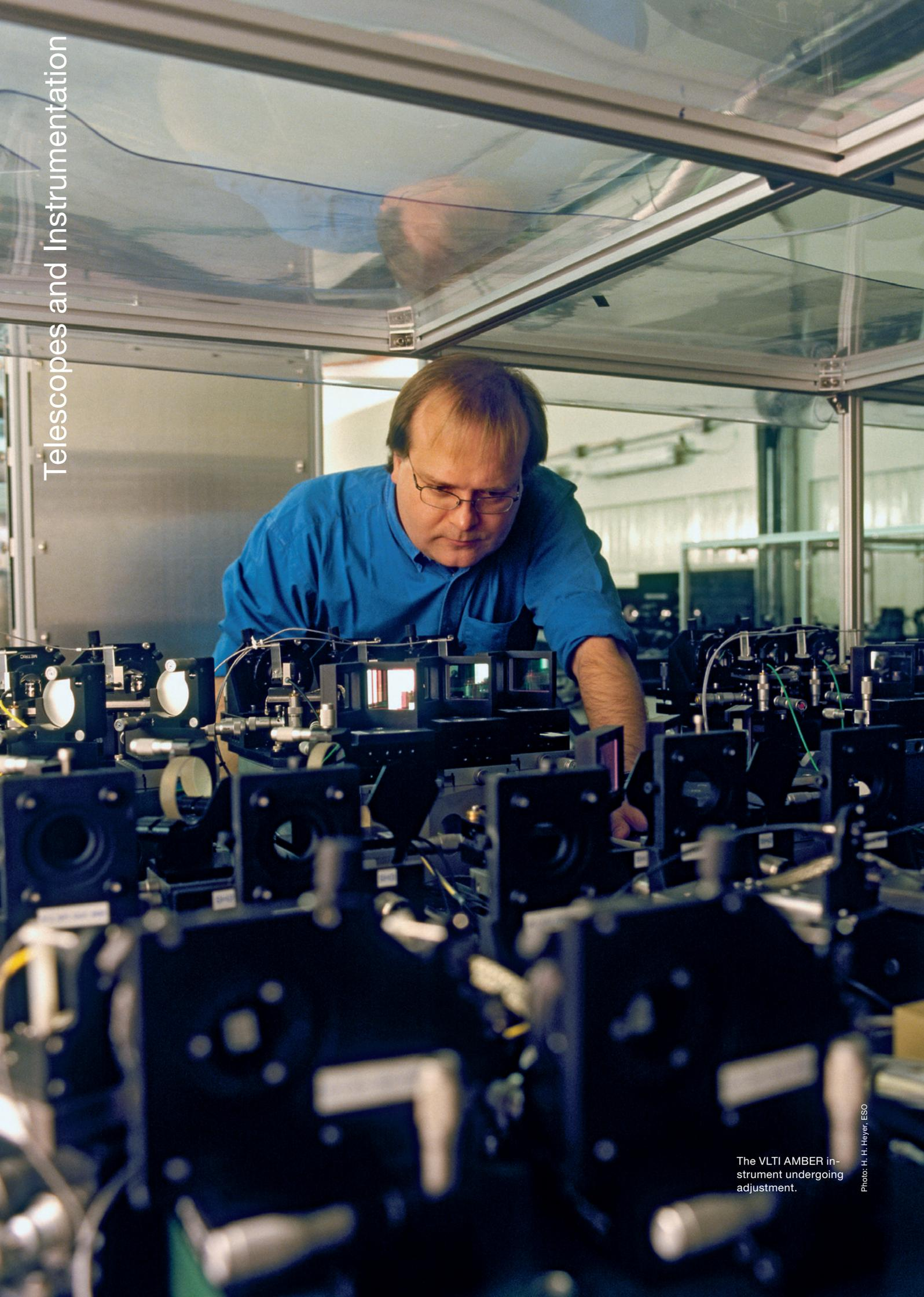
The VLT AMBER instrument undergoing adjustment.
