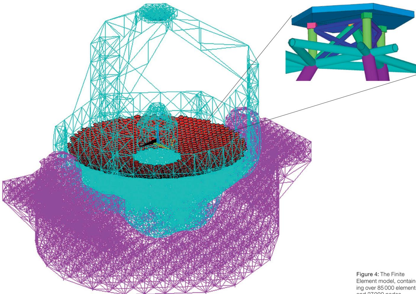
Figure 4: The Finite Element model, containing over 85 000 elements and 27 000 nodes.
