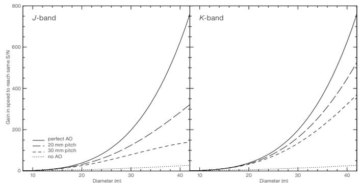
**Figure 7:** Gain in speed to achieve the same S/N compared with an 8-m telescope. The total number of actuators available at each diameter is kept constant and equal to the two technologies studied for the five-mirror solution.
