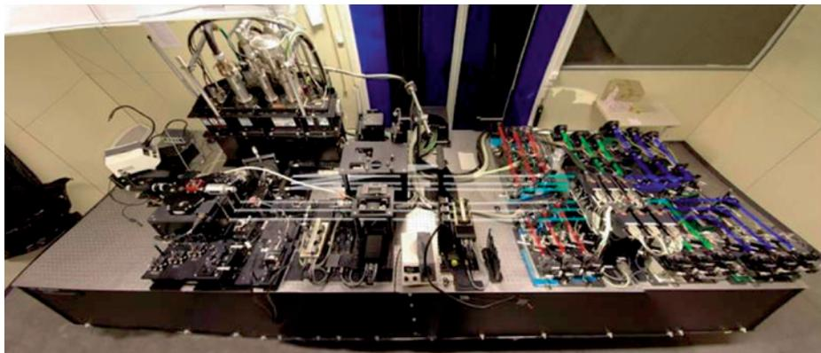
Figure 1: The VLTI instrument AMBER, which is the near-infrared instrument to combine and spectrally analyse the light caught by three of the telescope
