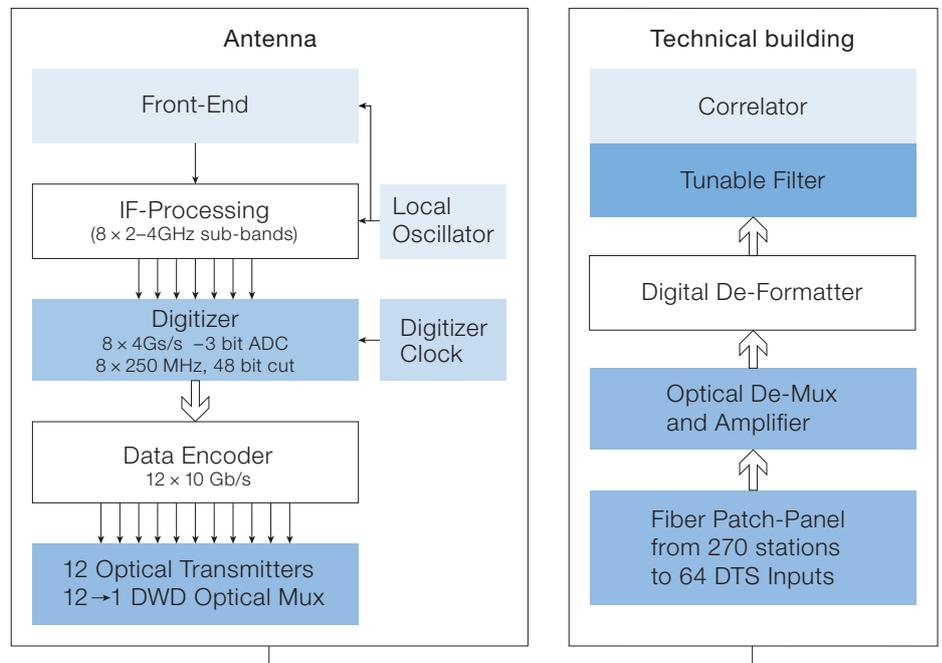
**Figure 2:** A schematic view of the ALMA system, showing the location of the Back-End subsystems between the Front-End receivers and the correlator. The Data Transmission System within the Back-End in the antenna processes, digitizes at 4 Gsamples/s and converts the 'low' frequency (4–12 GHz) signals output by the Front-End re-
