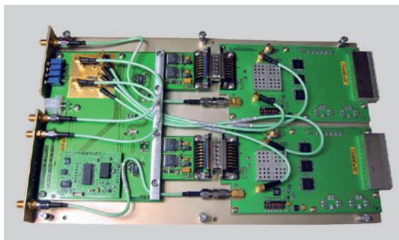
**Figure 3:** The Digitizer Assembly contains two VEGA digitizer chips (enclosed in the small metal boxes) and six PHOBOS de-multiplexer chips (the square black devices on the right side). The Digitizer Assembly converts two 2–4 GHz pass-band signals sampled at 4 Gsample/s into six 16-bit parallel streams at 250 MHz. The left side of the assembly contains the power supplies, the clocks distribution circuits and the low frequency circuits for communication and remote control.
