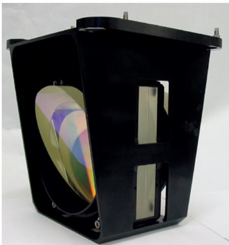
anti-reflection coated, 4k x 2k pixel CCD. VIMOS operates in three different modes: Imaging (IMG), Multi-Object Spectroscopy (MOS), and with Integral Field Unit (IFU). For a summary of the instrument capability and performance, see <http://www.eso.org/instruments/vimos/>
