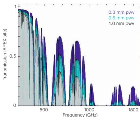
**Figure 2:** Zenith transmission of the atmosphere above Llano de Chajnantor at submillimetre wavelengths. Using data from the ALMA site characterisation, we calculate the 50 and 25 % quartile columns of precipitable water to 1.0 and 0.6 mm, respectively – excluding data taken during the Bolivian winter months (day numbers 15–90). The dark blue figure corresponds to 0.3 mm pwv, a rare, but not uncommon event that opens up the supra-THz windows.
