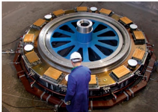
Figure 7b: Details of the hydrostatic system.
