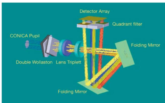
Figure 2: SDI optical concept. A double Wollaston prism splits the beam into four which are imaged through different filters located on the either side of the *H*-band methane feature at 1.62  $\mu\text{m}$ .
