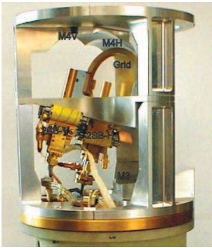
Figure 5: Photo of the cold optics assembly, with the two 2SB mixers.
