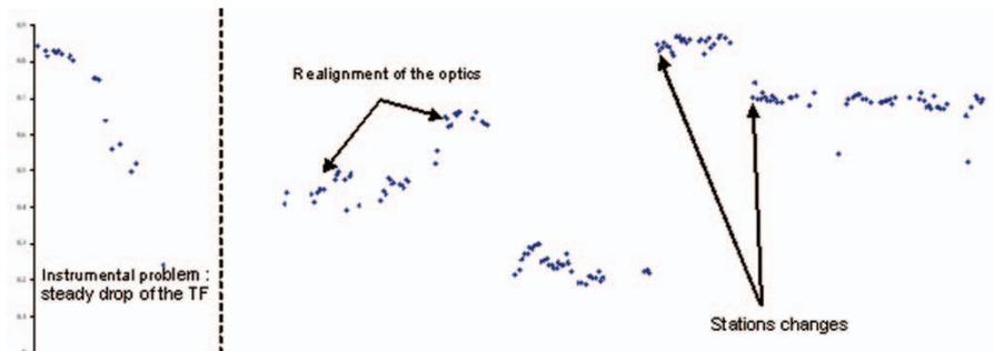
**Figure 5:** The instrumental transfer function for the commissioning instrument VINCI is shown for selected periods. Each dot represents a night of measurements on selected calibrators. The large jumps illustrate changes in the instrument configuration, while the small variations from one night to the next are due to atmospheric fluctuations.
