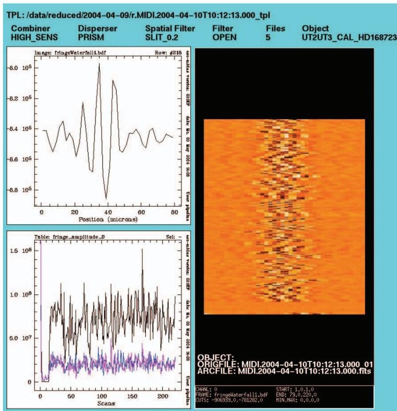
**Figure 3:** MIDI waterfall display. This example of the output display illustrates three components. The image on the right-hand-side is the so-called ‘waterfall display’ which shows the fringes in the entire data. The diagram on the top left-hand corner displays the central fringe and the one on the bottom left-hand corner is the result of the fringe amplitudes for the entire scan.
