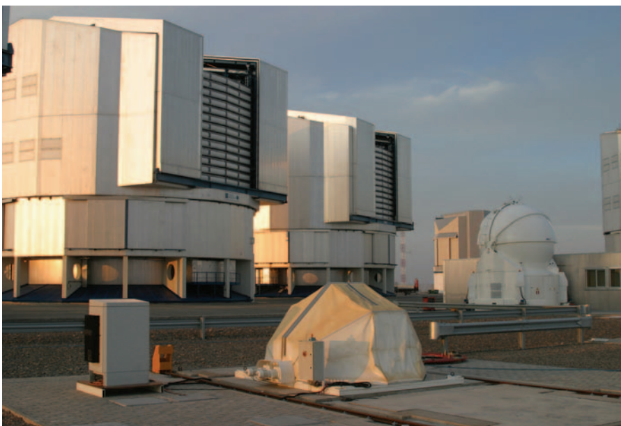
The enlarged telescope family with a VLTI Siderostat (foreground), the first VLTI Auxiliary Telescope (next to the VLTI building), three of the four Unit Telescopes and the VST enclosure (background). Photo: P. Kervella.
