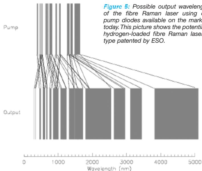
**Figure 5:** Possible output wavelengths out of the fibre Raman laser using different pump diodes available on the market as of today. This picture shows the potentiality of a hydrogen-loaded fibre Raman laser of the type patented by ESO.
