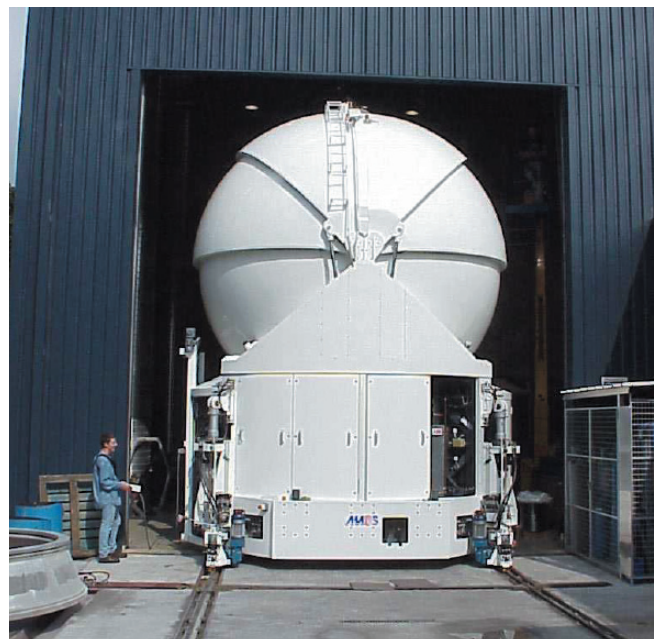
Figure 7: The first Transporter sees the sun light for the first time at AMOS (Liège, Belgium) during its functional tests last October. A dummy station will permit testing of the telescope on the sky before shipment to Paranal.
