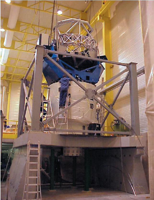
Figure 5: The first telescope on its test bench inside the dedicated hall at AMOS. In addition to tests at component level such as optical quality of each mirror, friction of the axis bearings, etc., the first telescope undergoes a thorough acceptance test programme including modal tests of the complete structure, dynamic response of the azimuth and altitude axis, OPL stability measurement, verification of structural deformation under gravity, pointing repeatability check and others.
