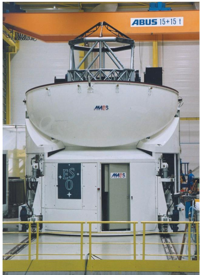
Figure 1: The first Auxiliary Telescope for the VLTI during final testing at AMOS in Liège (Belgium).
