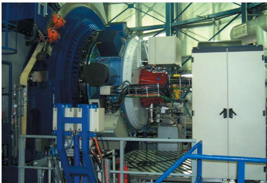
Figure 1: NAOS (light blue) and CONICA (red) attached to the Nasmyth B adapter of Yepun/UT4.
