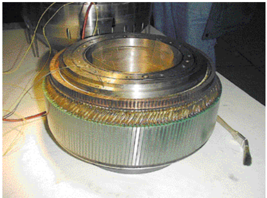
Figure 2: The faulty coil removed from the motor; the brush on the right gives the scale of this 60 kg piece.
