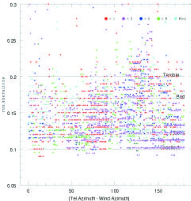
Figure 3a represents the "fitting" residual variations (non-modelised 7 first aberrations) of the image quality with NTT dome position relative to the wind direction as well as the wind speed. Colour code of wind speed is at top of figure in m/s.
