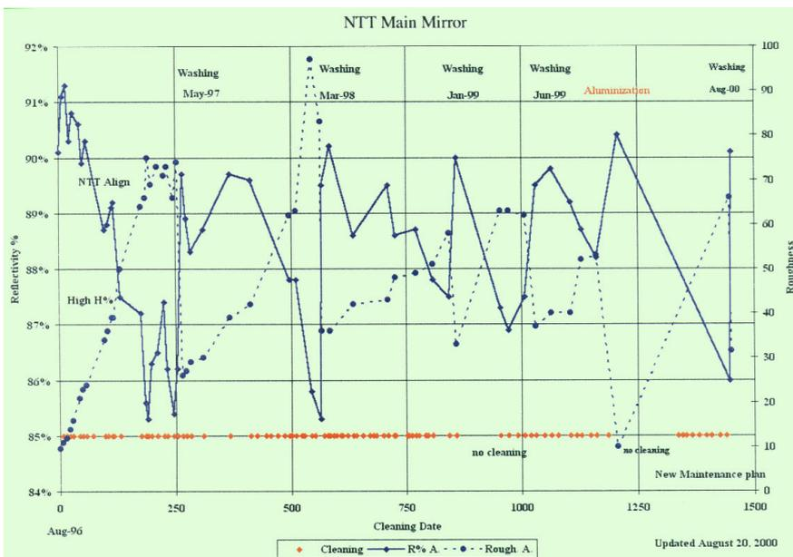
Figure 1: The variation of the reflectivity (R%) and roughness of the NTT main mirror during the period from August 1996 to August 2000.
