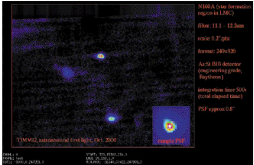
Figure 5: Image of the LMC star-formation region N160A. This was one of the first integrations on a scientifically interesting target with TIMMI2. The residual stripiness is due to grounding problems. While in principle this could be easily removed by Fourier filtering of the data, the cause is understood and the ground-loop problem will be solved while this article goes into print. The insert shows at a magnified scale a typical point-spread-function.
