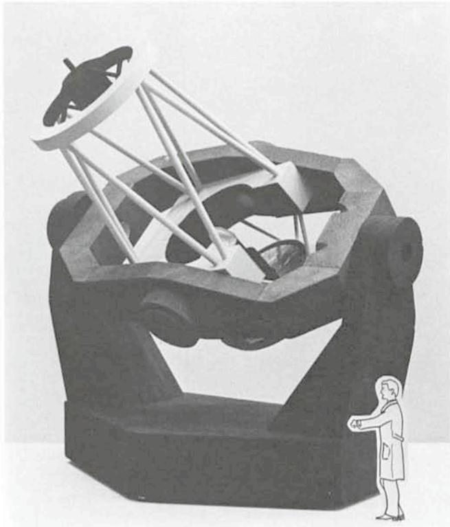
Fig. 1. — Model photo of the coude auxiliary telescope.
