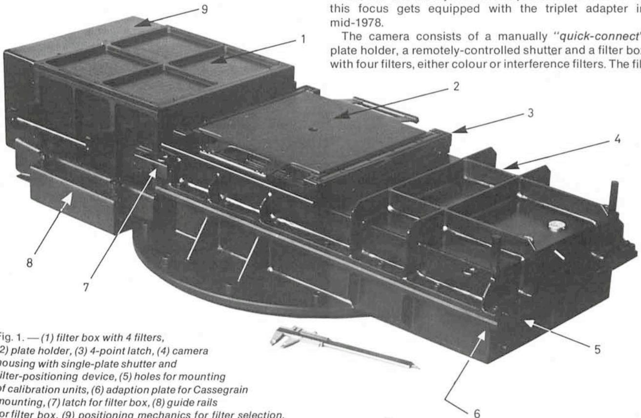
Fig. 1. — (1) filter box with 4 filters, (2) plate holder, (3) 4-point latch, (4) camera housing with single-plate shutter and filter-positioning device, (5) holes for mounting of calibration units, (6) adaption plate for Cassegrain mounting, (7) latch for filter box, (8) guide rails for filter box, (9) positioning mechanics for filter selection.
