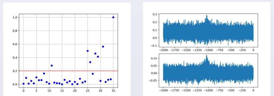
Example of anomaly detection among spectral sub-scans. Scores higher than 0.2 are classified as outliers. On the right, averaged anomalies (top) and normal cases (bottom) are shown, suggesting a slightly worse definition of the astronomical line in cases.
