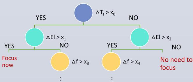
Thresholds  $x_0, x_1, x_2, \dots$  for all nodes can be adjusted to optimal values based on the running history of focus variation measurements together with the record of the corresponding features. Similar trees can be designed for pointing scans based on features like positional variations. These can also be adjusted with the running quality of the pointing model in place.
