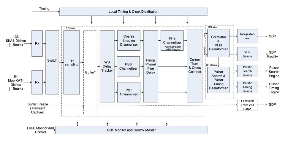
Note that Fringe Phase/Fine Delay has been moved to the Resampler for higher precision and signal fidelity
