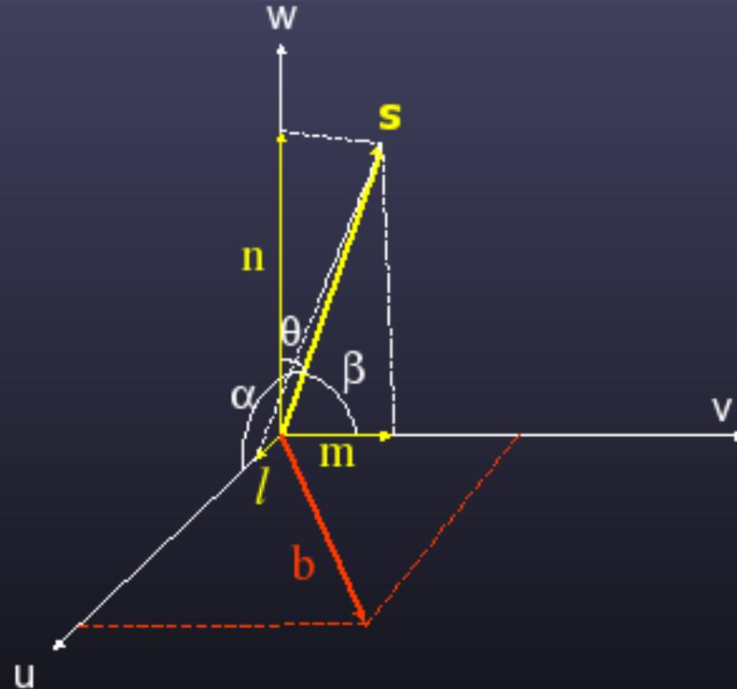
The baseline vector **b** is specified by its coordinates (u,v,w) (measured in wavelengths). In this special case,
