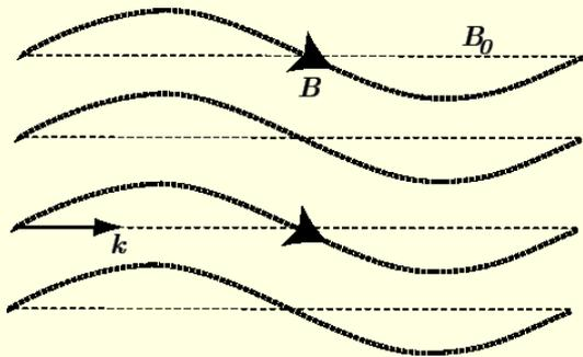
$$V_{Alf} = \sqrt{\frac{B^2}{4\pi\rho}} \quad \partial V_{Alf} = \sqrt{\frac{\partial B^2}{4\pi\rho}}$$
