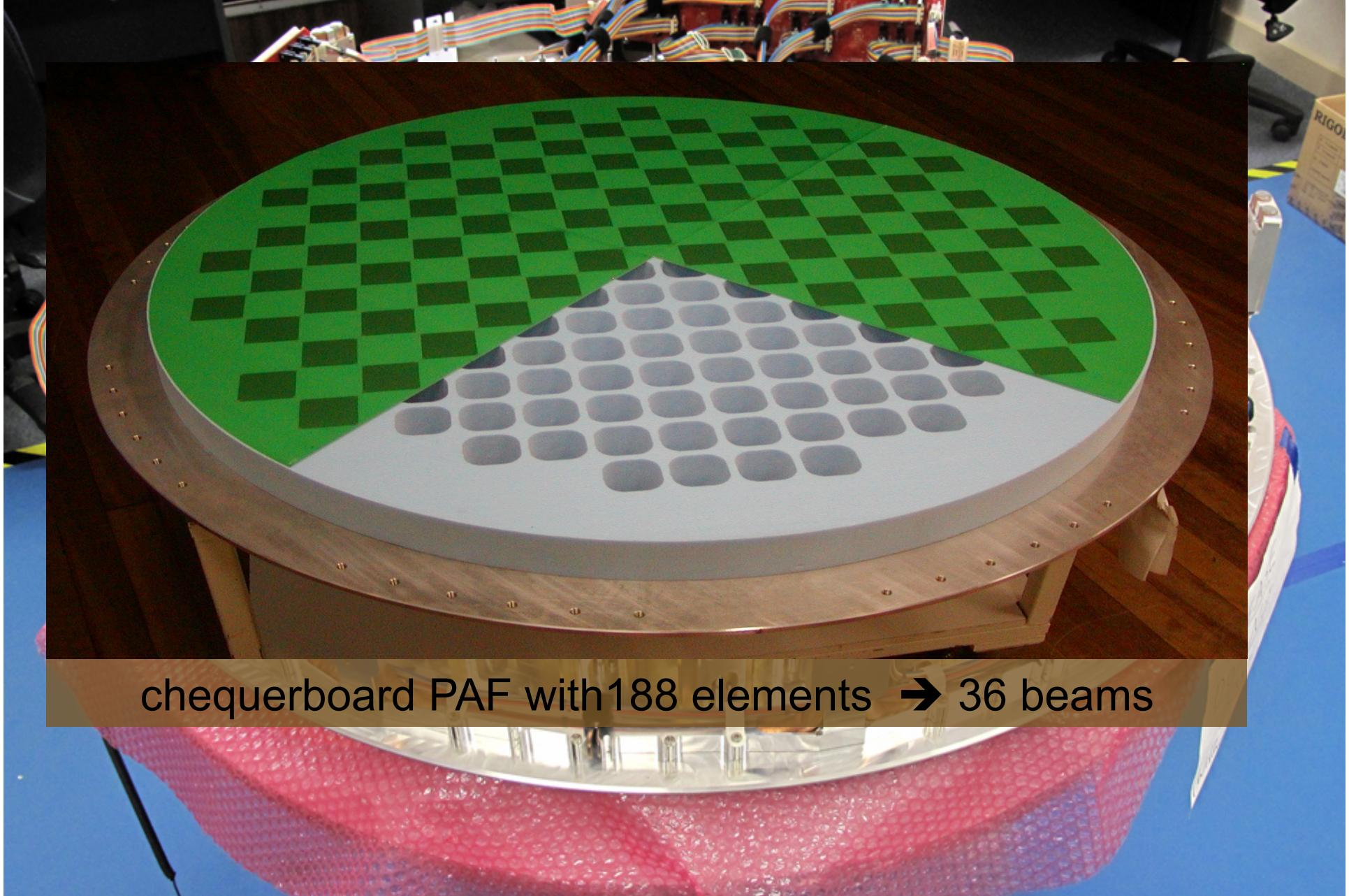
chequerboard PAF with 188 elements → 36 beams
