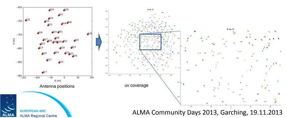
An interferometer does not record an image of the sky, but samples visibilities over a set of baselines defined by the antenna positions.
