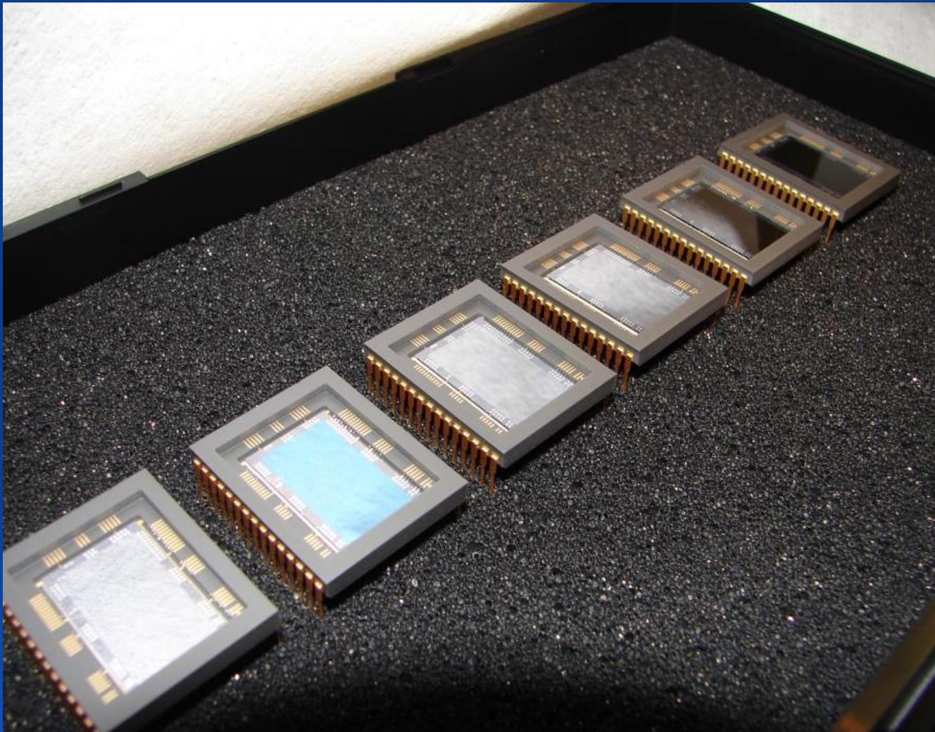
Six R-grade e2v CCD97's from the bonded, thinned, delta-doped wafer 18 have been packaged, wire-bonded and are being tested. One is AR coated with the FIREBALL multilayer design
