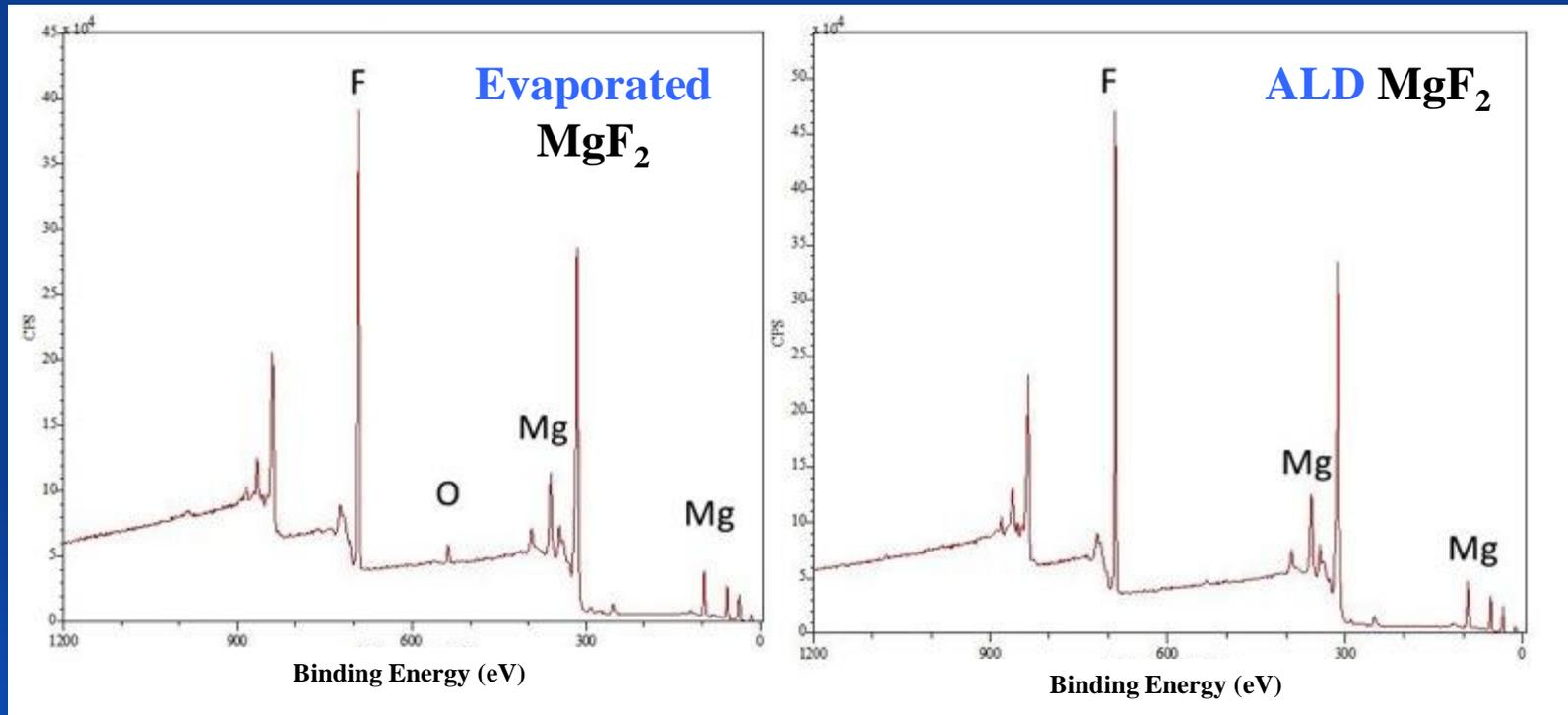
ALD  $\text{MgF}_2$  yields similar film stoichiometry to a thermally evaporated film, but with higher resistance to oxidation after air exposure.
