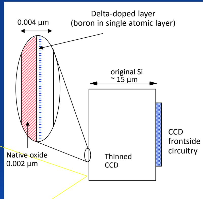
Low temperature process, compatible with VLSI, fully - fabricated devices (CCDs, CMOS, PIN arrays)
