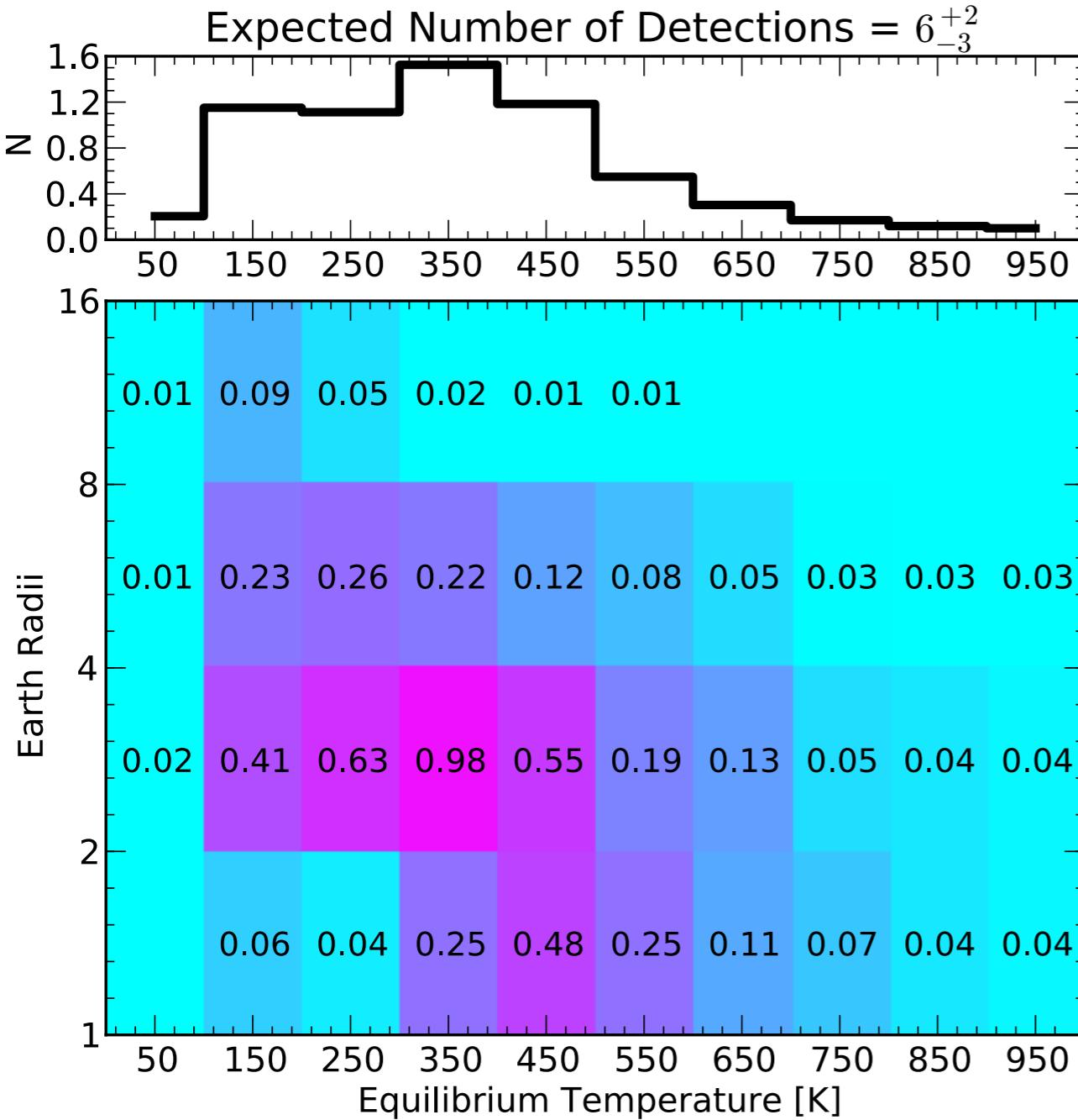
Simulated planet population (based on Kepler results) expected to be detectable by METIS direct imaging as a function of planetary radius and equilibrium temperature
