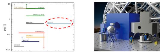
Left: METIS is the only E-ELT instrument which covers the thermal/mid-infrared wavelength range. Right: METIS at the NAsmyth platform of the E-ELT. Also shown are the cryostat support structure, the rig and the location of the electronics racks.
