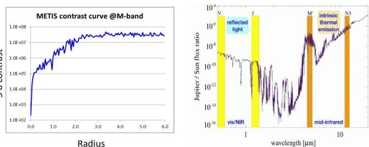
Left: Achievable 5- $\sigma$  radial contrast curves for an A0V star at 10 parsecs observed with METIS at M-band over one hour. Right: Much reduced star-planet contrast in the thermal infrared.
