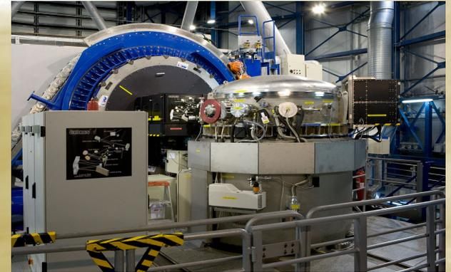
The detectors are four Aladdin III InSb arrays. A MACAO system for optimizing the *SNR* and the spatial resolution
