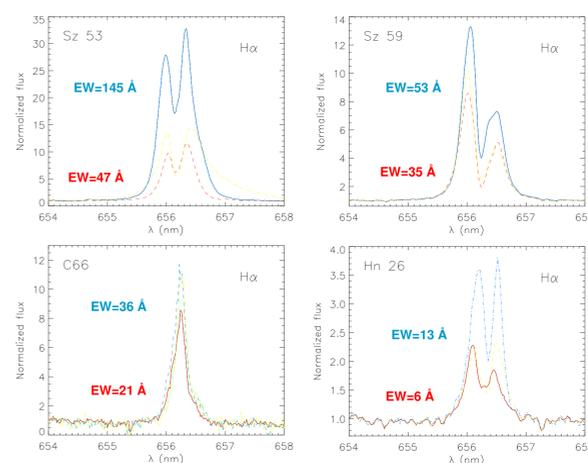
Fig. 3 – H $\alpha$  profile variations of four stars. The fluxes are normalized to the continuum. Each star was observed 3-4 times during two days (see different line colors and styles). The variations in line intensity, profile, and equivalent width are evident.
