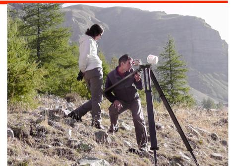
**Middle:** 2 tripods with 16 m baseline, part of an effective diluted aperture 57 m in diameter on the ground, are located on a sphere 200 meters in radius. The gondola is 100 m above the valley, at the focus surface later. **Right:** Aligning the mirror on its segment. **Left:** A close view on the tripod's head showing the mirror's supporting screws for tip, tilt and position adjustment.
