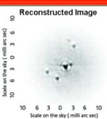
Numerical simulations from (3). Photon limited speckle masking results of a group of 6 stars from turbulent degraded interferograms with 50 mirrors aperturer with aperture rotation through night for 8 hours.
