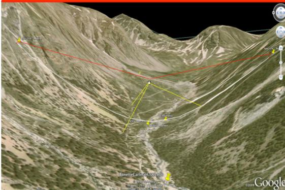
**Left:** Google Earth view of the Moutière valley where the prototype of the Carlina hypertelescope is under construction. The focal gondola, **(right)** will be suspended above the valley from a cable (red) attached to the South and North cliffs. The variable position and attitude of the gondola for tracking the star are controlled by 3 sets of motorized guy wires (yellow).
