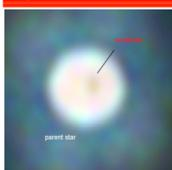
Exoplanet transit cross resolved star, as imaged by a 20 mirror cophased hypertelescope with a 100 m baseline. The star disk is 27 resels while the planet is 3 resels. (Courtesy Surya (4)).
