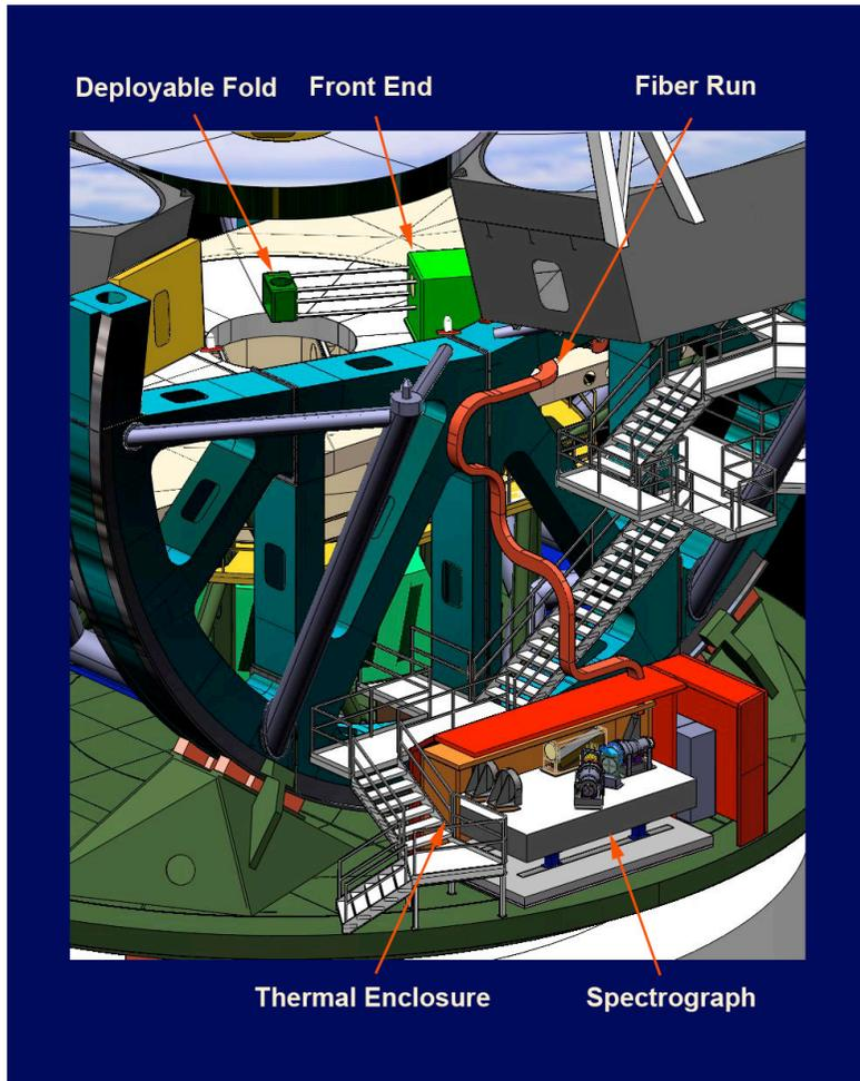
High-dispersion and precision radial velocity optical spectrograph
