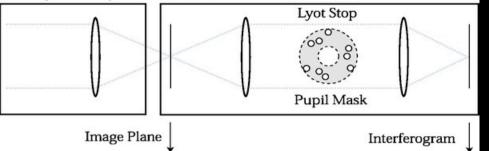
Placing an aperture mask in the pupil plane allows calibration of atmospheric turbulence on scales larger than the subapertures. Coupled with AO (for overall wavefront stabilization), it filters almost all noise from turbulence and AO errors. This yields very stable performance.
