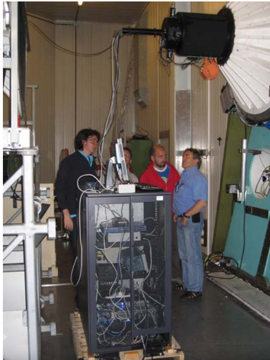
Figure 7. Iqueye installed at the NTT telescope in January 2009. The instrument is the black box attached to the Nasmyth focus, while the control electronics and rubidium clock are in the cabinet in the foreground.
