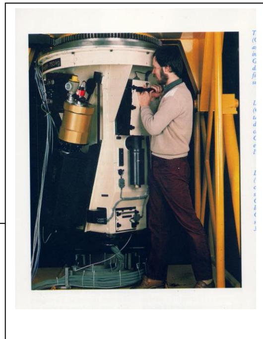
**Fig.1:** (a) The 3.6m telescope in la Silla (photo by Serge Brunner) and (b) the CASPEC spectrograph being tested in the laboratory by a young J.L. Lizon in 1982. The golden CCD cryostat is mounted on the left side of the instrument.
