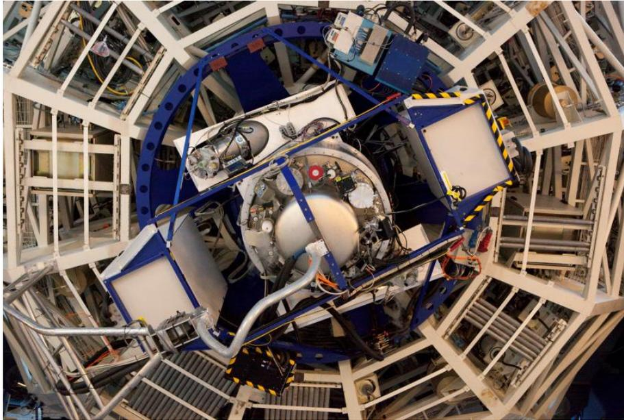
**Fig.4:** The three arm X-shooter instrument at the Cassegrain focus of the Kueyen telescope at the Paranal Observatory. At the center the NIR arm vessel, on the top the UV spectrograph with its CCD detector cryostat, at the bottom, partly hidden, the VIS spectrograph.
