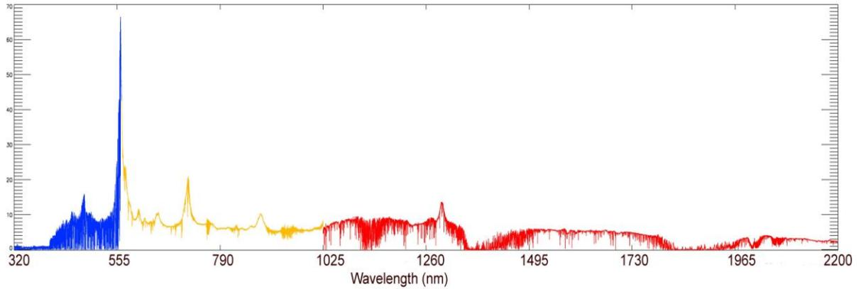
**Fig. 6:** Spectrum of the lensed QSO B1422+231 from the combination of four parallel 1200s exposures in the three arms of the instrument (Christensen and D’Odorico, in preparation). The blue part of the spectrum shows the UVB, the green the VIS, and the red the NIR data in relative flux units. The spectra are sky-subtracted but not corrected for telluric absorption. The resolving power is in 6200, 11000 and 8100 in the UVB, VIS and NIR arms respectively.
