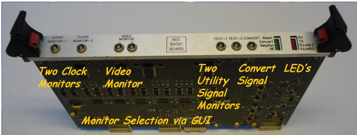
Figure 2 Front Panel NGC Basic Board
