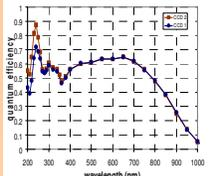
Figure 3. UVIS quantum efficiency
