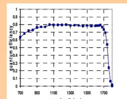
Figure 7. IR quantum efficiency
