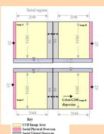
Figure 1. CCD readout configuration
