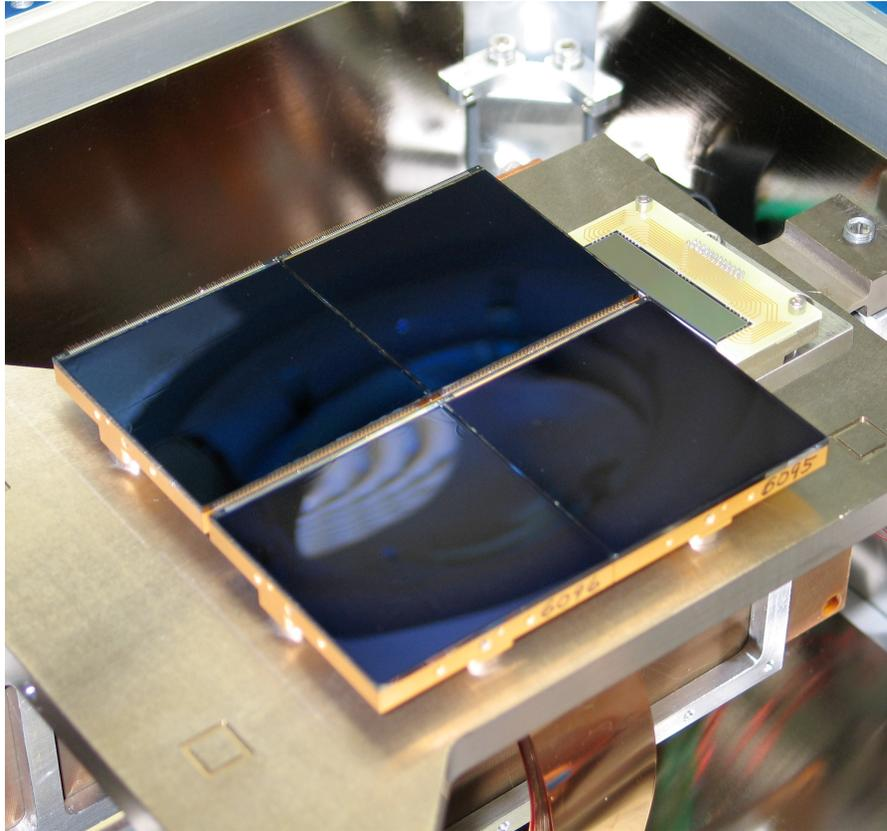
The image above shows four OTAs installed on the QUOTA focal plane. The image to the right is 120 sec exposure of M15 in the SDSS r' filter, taken 31 July 2008 using QUOTA. This image has overscan subtraction done, but no other post-processing.
