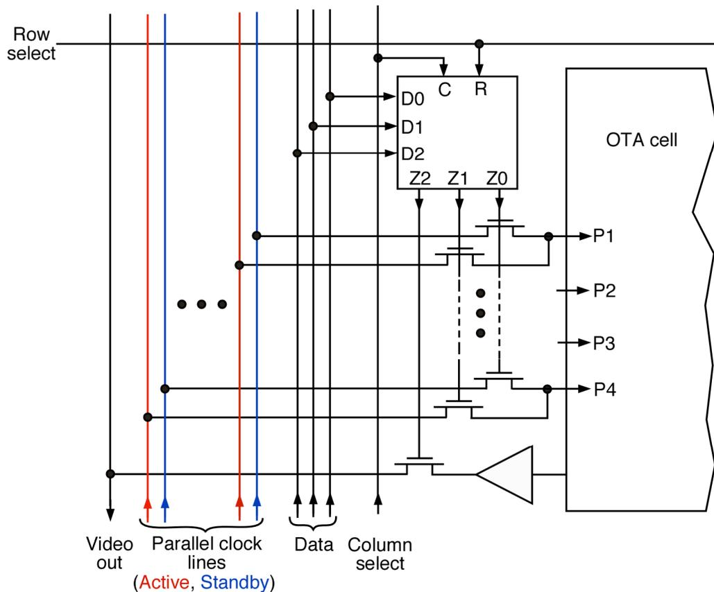
The parallel clocks have two states, active and standby, that are controlled through logic circuitry on the CCD. When a cell is in the active state the parallel clocks are connected to the clock drivers P1-P4. When in the standby state, the cell has the clock phases held in the charge collection state (P1=P4=Low voltage PL, P2=P3=High voltage PH).
