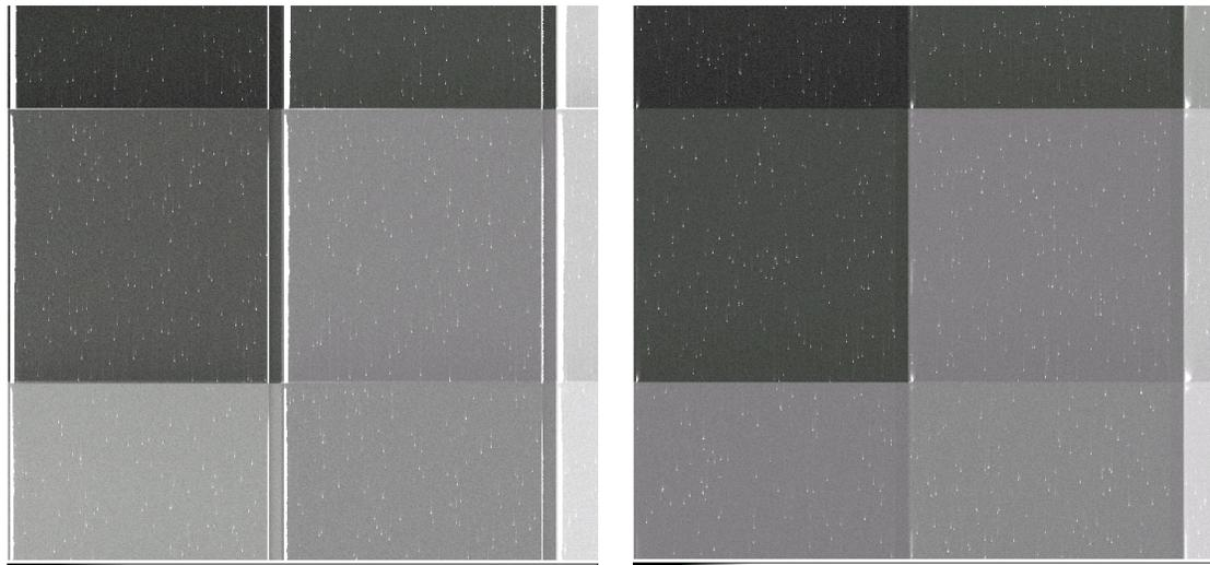
Images of OTA science cells showing the excess charge along the beginning columns of each cell that develops when the parallel clock high voltage is set to the OT shift optimization levels (10V) during science read out. The image on the right has PH reduced by 1V.
