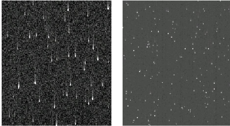
X-Ray images showing the effect of changing the high voltage setting of the parallel clocks (PH) on the vertical charge transfer efficiency. The image on the left has PH set to 11V, the image on the right has PH set to 8V.
