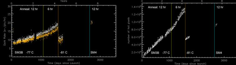
Figure 1: At left, the mean dark current (e-/pix/hr/yr) over time, illustrating the effect of reducing the operating temperature from  $-77$  C to  $-81$  C, and the rate following the 28-month period between ACS failure and repair. At right, the same trends for the growth of hot pixels.
