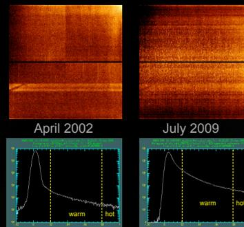
Figure 3: A comparison of dark images (above) obtained shortly after ACS installation in 2002, and following the repair in 2009. The brightening near the chip gap reflects the cumulative effects of hot pixel CTE tails far from the readout amps, and a horizontal striping feature from the new electronics (not a dark feature) is evident. Corresponding histograms (bottom) indicate the growing population of warm and hot pixels over this period.
