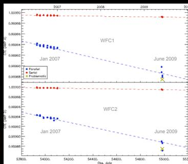
Figure 2: Parallel (blue) and serial (red) CTE as measured by the EPER test at one signal level (1620e), showing post-SM4 results to be near extrapolations from January 2007
