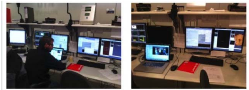
Figure 7: the pictures show the duplication of the main displays (instrument workstation, observing and data management consoles) to the Remote Access Facility (RAF): in ESO-Santiago premises allowing collaborative work between staff located at Paranal and colleagues in Santiago.
