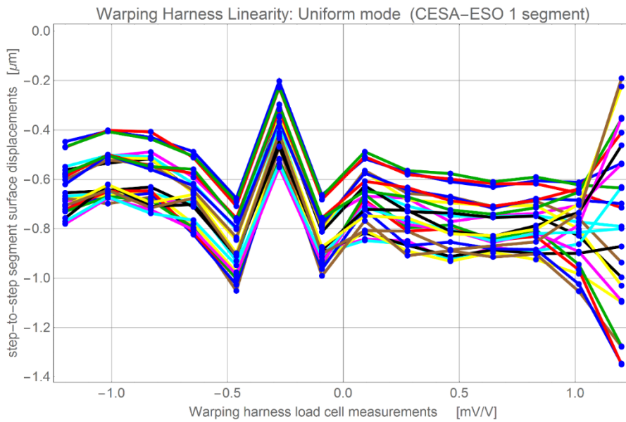
Figure 27. Ramp test with uniform actuation pattern
