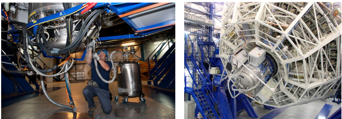
Figure 3: Examples of LIN cooled instruments at VLT: X-shooter LIN refilling from portable dewar and transfer line (left), VLT 8-m mirror cell with SINFONI attached at Cassegrain focus (right).
