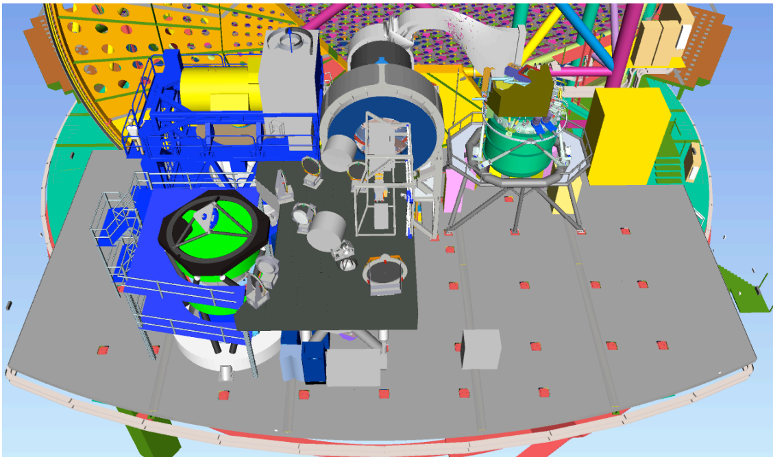
Figure 10. Snapshot of the ELT 3D model showing a view of Nasmyth A with the instruments and the Pre-Focal Station.
