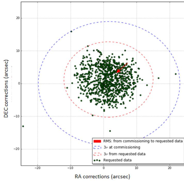
Figure 5: UT1 guide star acquisition accuracy, first quarter 2018
