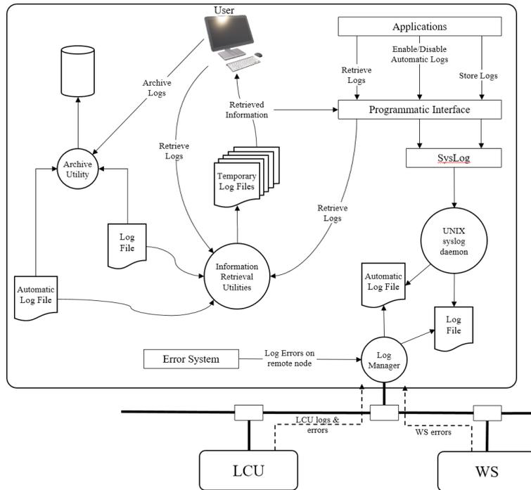
Figure 2: Logging system architecture
