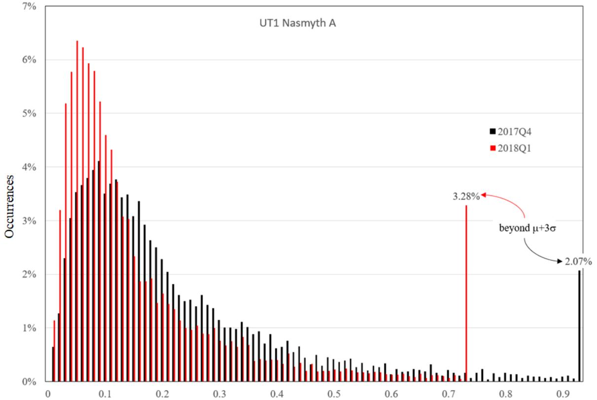
Field stabilization correction RMS over a minute as measured on a great circle of the celestial sphere (arcsec)
