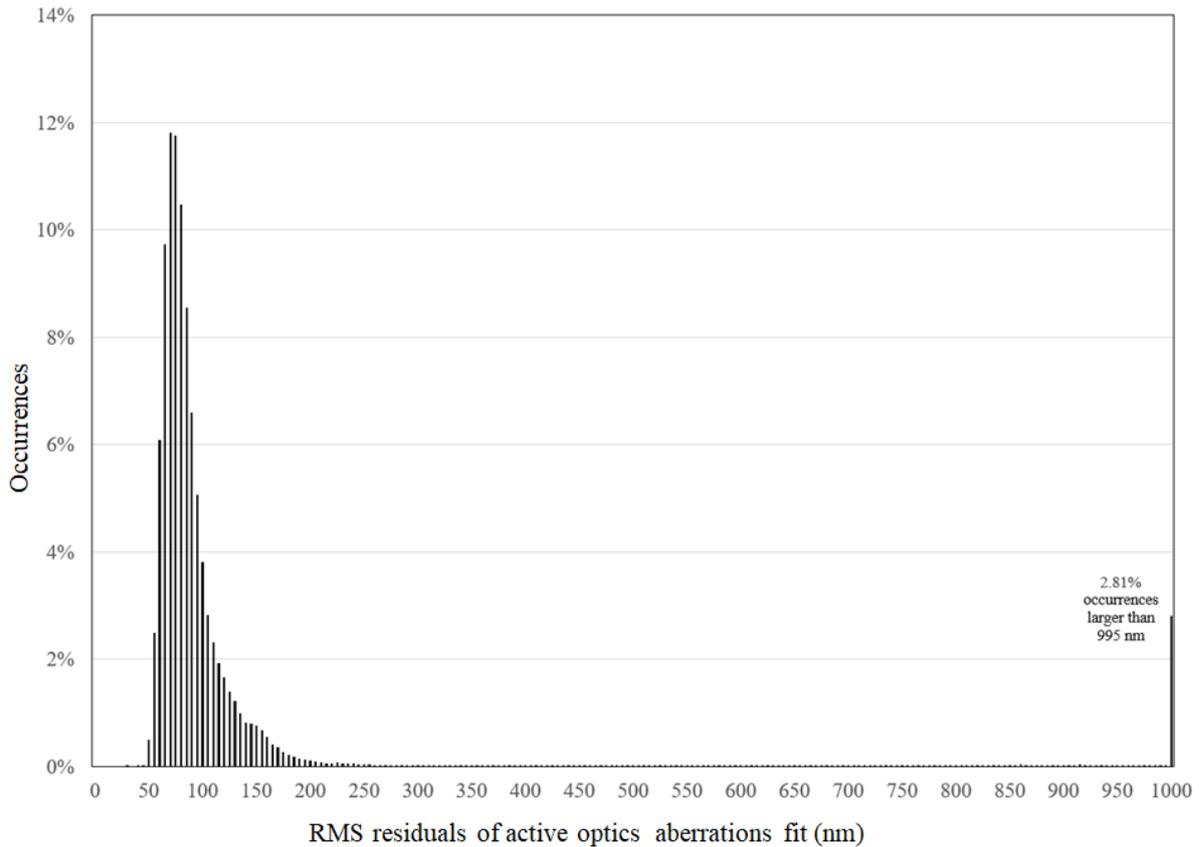
Figure 14: UT1 active optics performance between May 2017 and April 2018 (the widening of the main peak to the right is due to the use of a more robust but less accurate wavefront reconstruction algorithm sometime required by specific circumstances)
