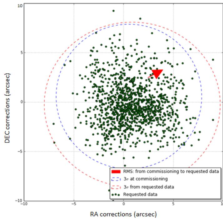
Figure 6: UT2 guide star acquisition accuracy, first quarter 2018
