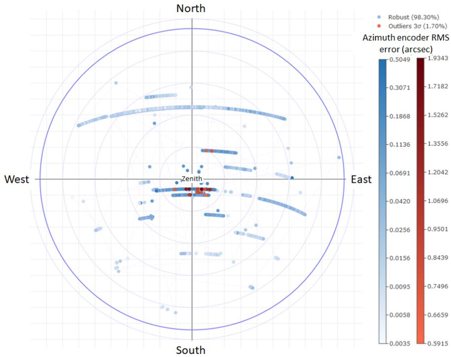
Figure 10: UT1 azimuth axis encoder error
