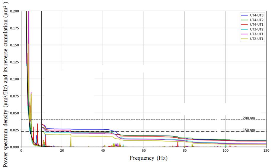
Figure 17: VLT baseline optical path difference: cumulative power density spectra during August 2017
