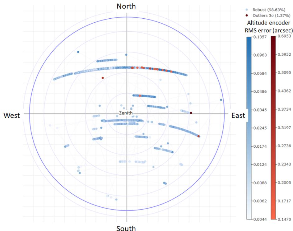
Figure 9: UT1 altitude axis encoder error
