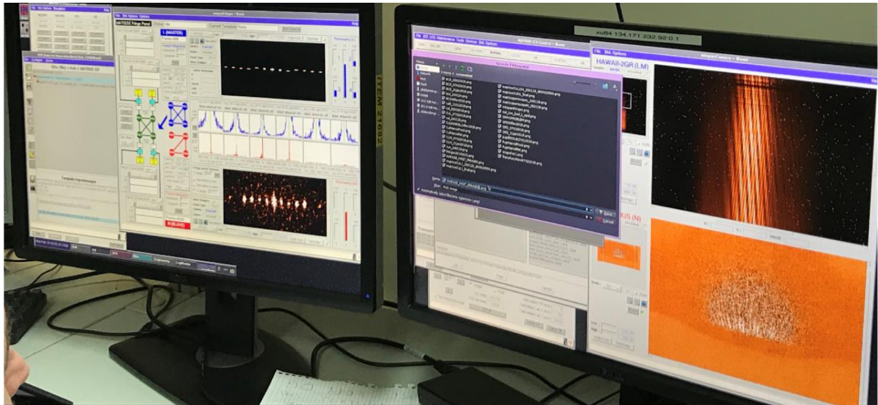
Figure 1: MATISSE control monitor. On the right screen, we see 4T dispersed fringes in the x\text{-}\lambda interferograms. Here the upper image shows medium resolution L band fringes on the Hawaii II detector and the lower image shows N band fringes in low spectral resolution. The left screen shows the fringe detection and tracking panel (right) and the “Broker of Observing Blocs” (BOB) at the extreme left. On the fringe detection panel, we see the six fringes peaks resulting from the 2D Fourier Transform of the x\text{-}\lambda interferograms (L is up, N is down). The position of the fringe peak for a given baseline yields the differential OPD (the piston) on this baseline. Here the fringes peaks are close to the central horizontal line, indicating that all pistons are close to zero.
