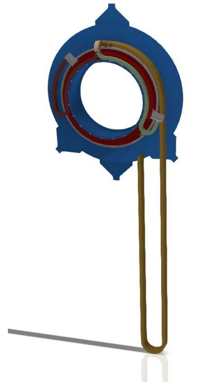
Figure 6: NGS Adapter: Cable Wrap System
