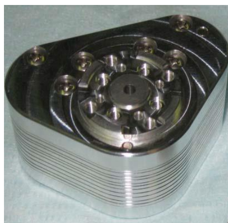
Figure 3. (a) OMT implemented in four plates at UChile. (b) OMT implemented in nine plates.
