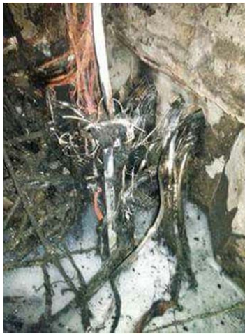
Figure 14 Burned cable in a vault in Santiago city center.
