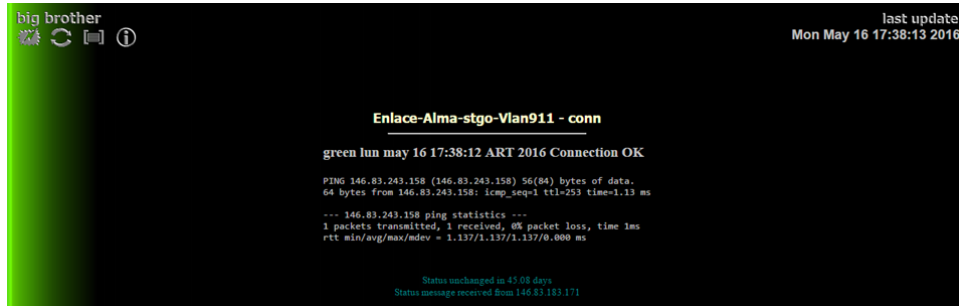
Figure 10 monitoring of the end-to-end functionality at IP level.
