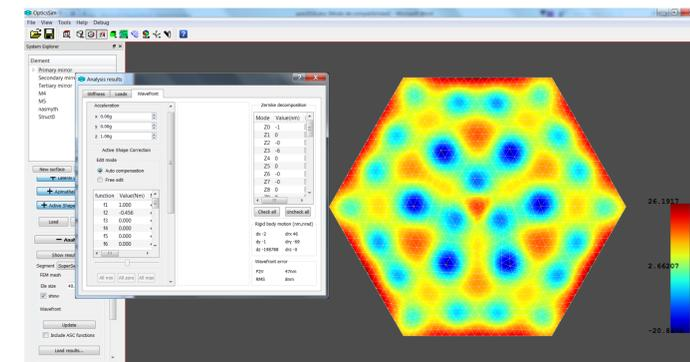
Fig. 10 Segmented mirror wavefront analysis
