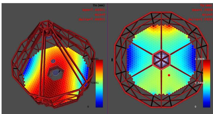
Fig. 3 FEM results. Deflection of Segmented mirror
